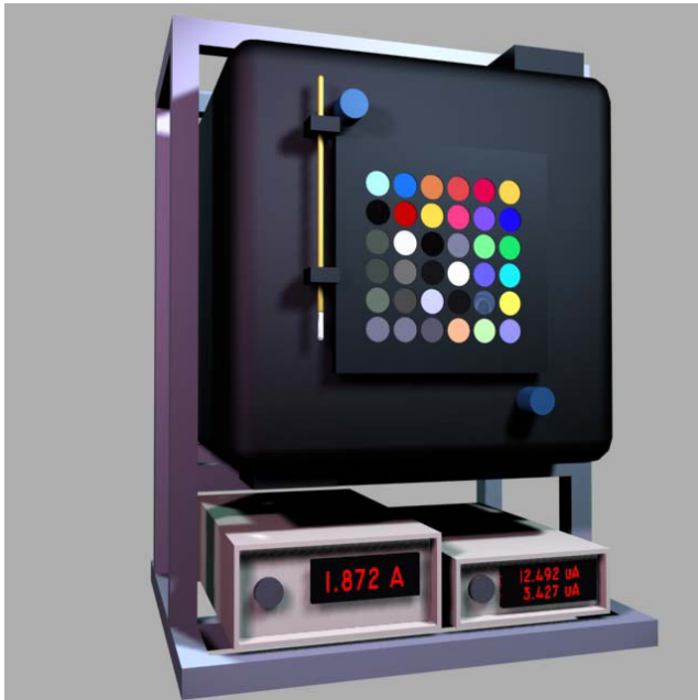
Figure 1. Each DMATS unit will consist of a uniform illumination source with a suite of optical targets mounted in a faceplate, power supply, monitoring devices, and a laptop computer for automatic data logging.
