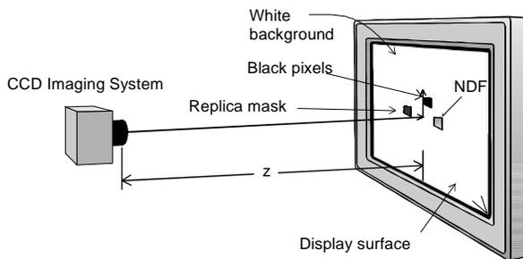
Figure 2. Measurement configuration.
